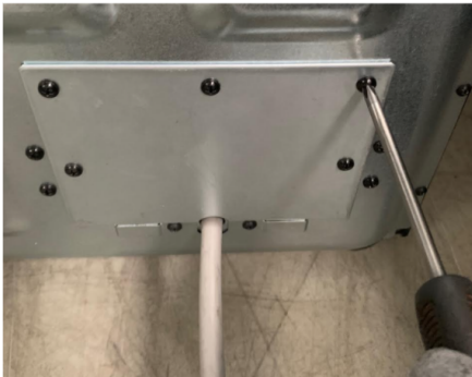
Assemble cover and tighten screws.
