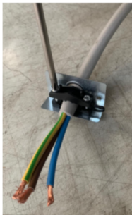
Fix power cord to the plastic holder.
